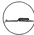
PITTSBURGH LOCK Pocket Depth: 1/2" Capacity: 16 Gauge Auxiliary
