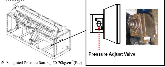
If pressure higher than this range, that would cause oil temperature rise up quickly.
